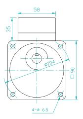
Motor Round Shaft with Terminal Box
